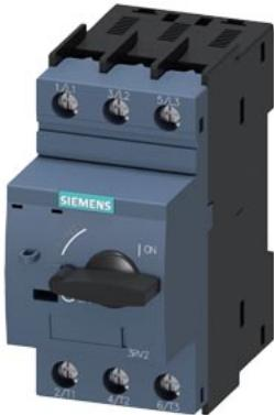
Circuit breaker size S0 for starter combination Rated current 20 A N-release 260 A screw terminal Standard switching capacity
