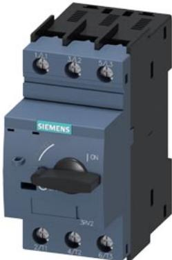
Circuit breaker size S0 for starter combination Rated current 1.6 A N-release 21 A screw terminal Standard switching capacity
