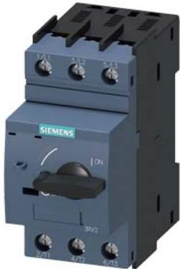
Circuit breaker size S00 for starter combination Rated current 1.6 A N-release 21 A screw terminal Standard switching capacity
