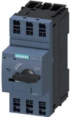
Circuit breaker size S00 for starter combination Rated current 0.8 A N-release 10 A Spring-type terminal Standard switching capacity
