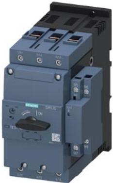
Circuit breaker size S3 for motor protection CLASS 10 with overload relay function
