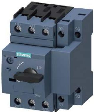
Circuit breaker size S00 for motor protection, CLASS 10 with overload relay function A-release 0.9...1.25 A N-release 16 A screw terminal Standard switching capacity
