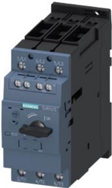
Special type Circuit breaker size S2 for motor protection, CLASS 10 A-release 35...45 A N-release 650 A screw terminal Standard switching capacity with transverse auxiliary switches 1 NO+1 NC Ambient temperature -50 °C 250 switching cycles
