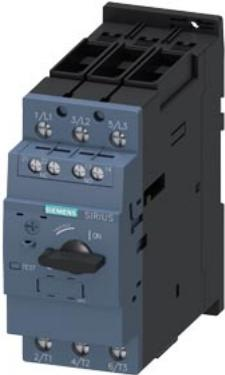
Circuit breaker size S2 for motor protection, CLASS 10 A-release 9.5...14 A N-release 208 A screw terminal Standard switching capacity with transverse auxiliary switches 1 NO+1 NC
