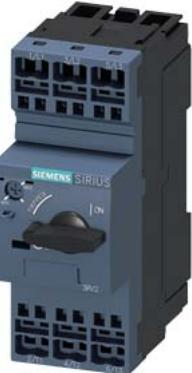
circuit breaker frame size S0 for motor protection, Class 10 thermal overload release 10...16 A short-circuit release 208 A spring-loaded terminal switching capacity 30 kA at 600 V according to UL/CSA
