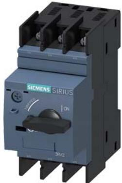
Circuit breaker size S0 for motor protection, CLASS 10 A-release 23...28 A N-release 364 A ring cable lug connection Standard switching capacity
