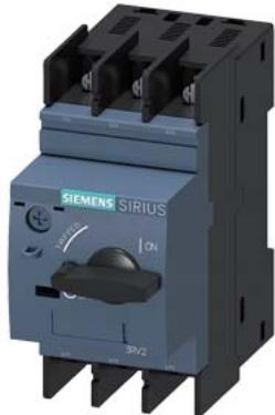
Circuit breaker size S0 for motor protection, CLASS 10 A-release 27...32 A N-release 400 A ring cable lug connection Standard switching capacity
