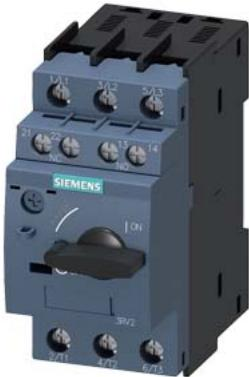
Circuit breaker size S0 for motor protection, CLASS 10 A-release 9...12.5 A N-release 163 A screw terminal Standard switching capacity with transverse auxiliary switches 1 NO+1 NC
