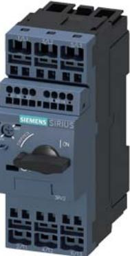
Circuit breaker size S0 for motor protection, CLASS 10 A-release 1.4...2 A N-release 26 A Spring-type terminal Standard switching capacity with transverse auxiliary switches 1 NO+1 NC
