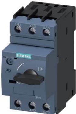
Circuit breaker size S0 for motor protection, CLASS 10 A-release 1.1...1.6 A N-release 21 A screw terminal Standard switching capacity
