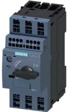
Circuit breaker size S00 for motor protection, CLASS 10 A-release 10...16 A N-release 208 A Spring-type terminal Standard switching capacity with transverse auxiliary switches 1 NO+1 NC
