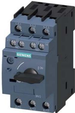
Circuit breaker size S00 for motor protection, CLASS 10 A-release 4.5...6.3 A N-release 82 A screw terminal Standard switching capacity with transverse auxiliary switches 1 NO+1 NC
