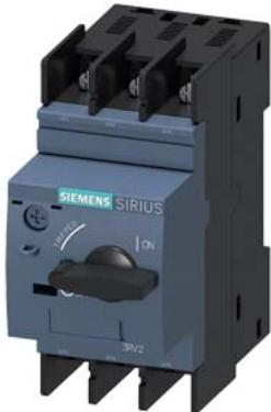
Circuit breaker size S00 for motor protection, CLASS 10 A-release 1.4...2 A N-release 26 A ring cable lug connection Standard switching capacity
