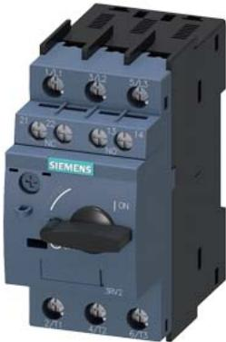
Circuit breaker size S00 for motor protection, CLASS 10 A-release 1.4...2 A N-release 26 A screw terminal Standard switching capacity with transverse auxiliary switches 1 NO+1 NC
