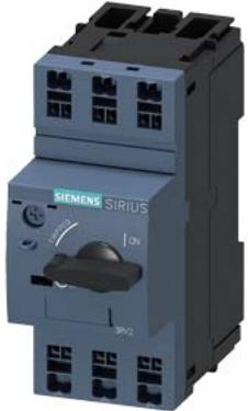
Circuit breaker size S00 for motor protection, CLASS 10 A-release 0.45...0.63 A N-release 8.2 A Spring-type terminal Standard switching capacity
