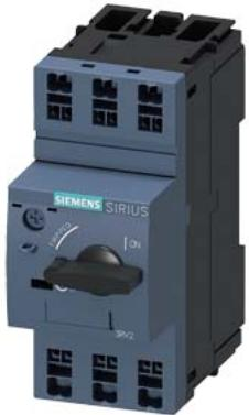
Circuit breaker size S00 for motor protection, CLASS 10 A-release 0.22...0.32 A N-release 4.2 A Spring-type terminal Standard switching capacity
