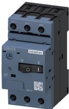
Circuit breaker size S00 for motor protection, CLASS 10 A-release 1.4...2 A N-release 26 A Screw terminal Standard switching capacity
