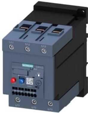
overload relay 70...90 A thermal for motor protection frame size S3, Class 10 stand-alone installation main circuit: screw auxiliary circuit: spring-loaded terminal manual-automatic RESET
