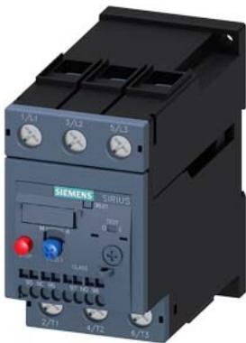
overload relay 28...40 A thermal for motor protection frame size S2, Class 10 stand-alone installation main circuit: screw auxiliary circuit: spring-loaded terminal manual-automatic RESET
