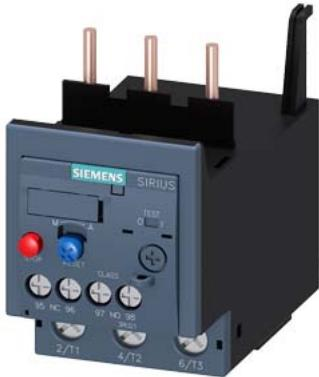
Overload relay 7...10 A Thermal For motor protection Size S2 Class 10 Contactor mounting Main circuit: screw terminal Auxiliary circuit: screw terminal Manual-Automatic-Reset
