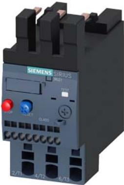
overload relay 14...20 A thermal for motor protection frame size S0, Class 10 for mounting on contactors main circuit: spring-loaded terminal auxiliary circuit: spring-loaded terminal manual-automatic RESET
