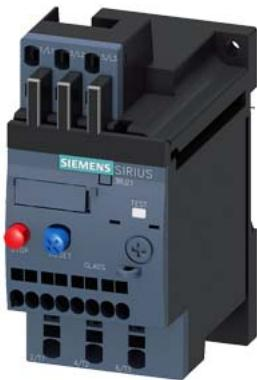
overload relay 1.4...2.0 A thermal for motor protection frame size S00, Class 10 stand-alone installation main circuit: spring-loaded terminal auxiliary circuit: spring-loaded terminal manual-automatic RESET
