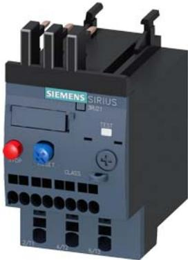
overload relay 0.35...0.50 A thermal for motor protection frame size S00, Class 10 for mounting on contactors main circuit: spring-loaded terminal auxiliary circuit: spring-loaded terminal manual-automatic RESET
