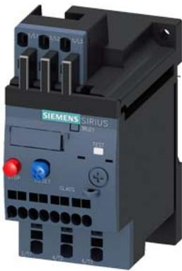
overload relay 0.22...0.32 A thermal for motor protection frame size S00, Class 10 stand-alone installation main circuit: spring-loaded terminal auxiliary circuit: spring-loaded terminal manual-automatic RESET
