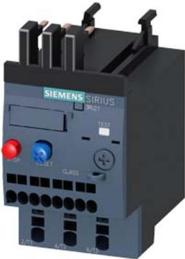
overload relay 0.18...0.25 A thermal for motor protection frame size S00, Class 10 for mounting on contactors main circuit: spring-loaded terminal auxiliary circuit: spring-loaded terminal manual-automatic RESET
