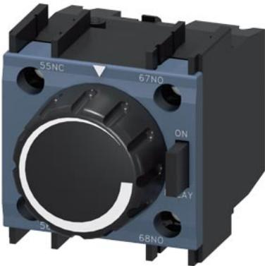
pneumatically time-delayed auxiliary switch, ON-delay, 1-30 s, 1 NO + 1 NC, for mounting to contactors 3RT202
