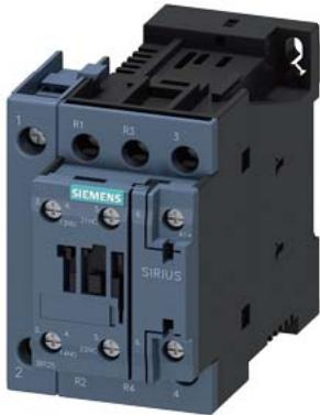
power contactor, AC-3, 25 A, 11 kW / 400 V, 4-pole, 24 V DC, main contacts: 2 NO + 2 NC, auxiliary contacts: 1 NO + 1 NC, screw terminal, size: S0
