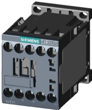
power contactor, AC-3, 12 A, 5.5 kW / 400 V, 4-pole, 220 V AC, 50 Hz / 240 V, 60 Hz, main contacts: 2 NO + 2 NC, screw terminal, size: S00
