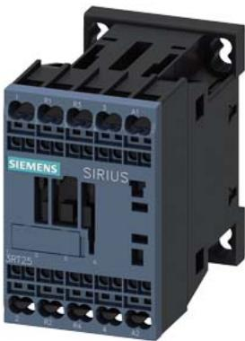
power contactor, AC-3, 9 A, 4 kW / 400 V, 4-pole, 230 V AC, 50/60 Hz, main contacts: 2 NO + 2 NC, spring-loaded terminal, size: S00
