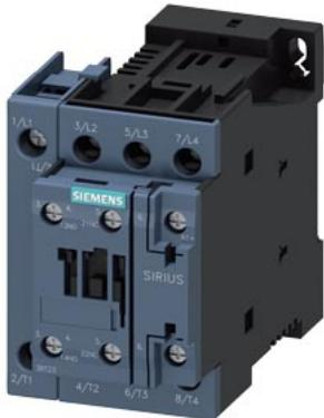
contactor AC-1, 35 A, 400 V / 40 °C, 4-pole, 24 V DC, auxiliary contacts: 1 NO + 1 NC, screw terminal, size: S0
