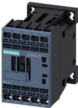
contactor AC-1, 18 A, 400 V / 40 °C, 4-pole, 24 V DC, spring-loaded terminal, size: S00
