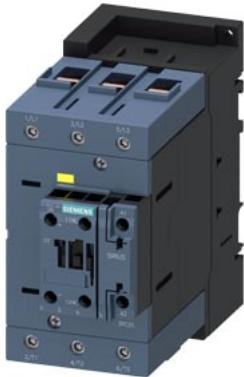
power contactor, AC-3e/AC-3, 110 A, 55 kW / 400 V, 3-pole, 83-150 V AC/DC, 50/60 Hz, with integrated varistor, auxiliary contacts: 1 NC, screw terminal, size: S3, F-PLC-IN
