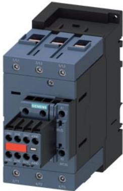
power contactor, AC-3e/AC-3, 110 A, 55 kW / 400 V, 3-pole, 20-33 V AC/DC, 50/60 Hz, with integrated varistor, auxiliary contacts: 2 NO + 2 NC, screw terminal, size: S3, captive auxiliary switch
