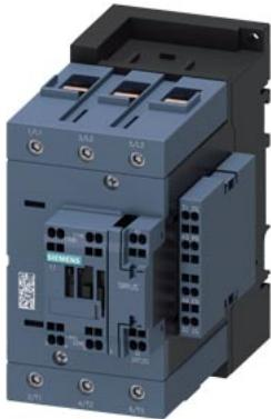
power contactor, AC-3e/AC-3, 80 A, 37 kW / 400 V, 3-pole, 230 V AC, 50 Hz, auxiliary contacts: 2 NO + 2 NC, main circuit: screw terminal, control and auxiliary circuit: spring-loaded terminal, size: S3, lateral auxiliary switch
