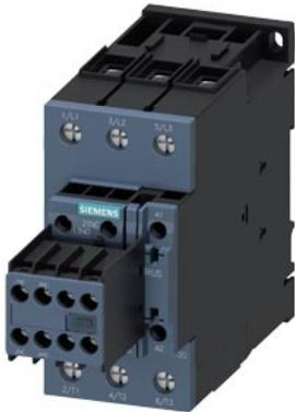
power contactor, AC-3e/AC-3, 65 A, 30 kW / 400 V, 3-pole, 20-33 V AC/DC, 50/60 Hz, with integrated varistor, auxiliary contacts: 2 NO + 2 NC, screw terminal, size: S2, removable auxiliary switch
