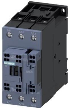
power contactor, AC-3e/AC-3, 51 A, 22 kW / 400 V, 3-pole, 20-33 V AC/DC, 50/60 Hz, with integrated varistor, auxiliary contacts: 1 NO + 1 NC, main circuit: screw terminal, control and auxiliary circuit: spring-loaded terminal, size: S2,
