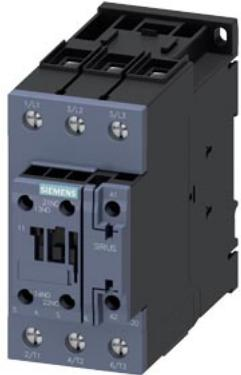
power contactor, AC-3e/AC-3, 51 A, 22 kW / 400 V, 3-pole, 20-33 V AC/DC, 50/60 Hz, with integrated varistor, auxiliary contacts: 1 NO + 1 NC, screw terminal, size: S2
