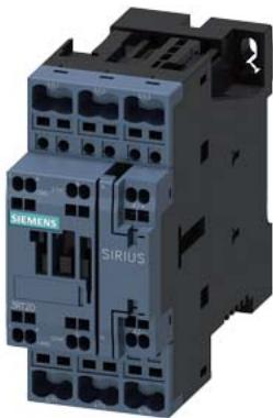
power contactor, AC-3e/AC-3, 25 A, 11 kW / 400 V, 3-pole, 24 V DC, auxiliary contacts: 1 NO + 1 NC, spring-loaded terminal, size: S0
