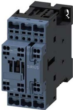
power contactor, AC-3e/AC-3, 25 A, 11 kW / 400 V, 3-pole, 24 V DC, auxiliary contacts: 1 NO + 1 NC, spring-loaded terminal, size: S0, communication-capable
