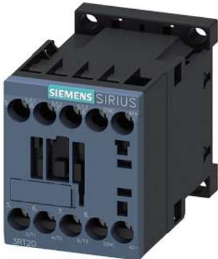
power contactor, AC-3e/AC-3, 9 A, 4 kW / 400 V, 3-pole, 110 V DC, auxiliary contacts: 1 NC, screw terminal, size: S00
