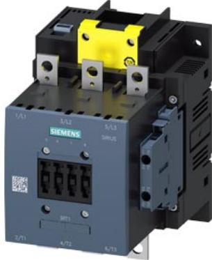
power contactor AC-1 275 A / 690 V / 40 °C 3-pole, Uc: 200-277 V AC(50-60 Hz) / DC F-PLC input 24 V DC drive: electronic auxiliary contacts 2 NO + 2 NC main circuit: busbar control and auxiliary circuit: screw terminal
