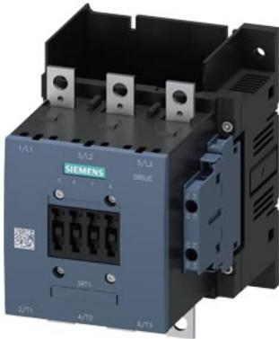
power contactor AC-1 275 A / 690 V / 40 °C 3-pole, drive: without auxiliary contacts
