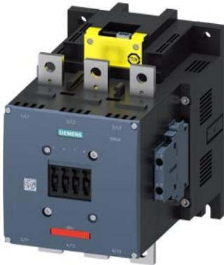
power contactor, AC-3e/AC-3 400 A, 200 kW / 400 V AC (50-60 Hz) / DC 96-127 V x (0.8-1.1) F-PLC input 24 V DC 3-pole, auxiliary contacts 2 NO + 2 NC permanently mounted drive: electronic main circuit: busbar control and auxiliary circuit: screw terminal
