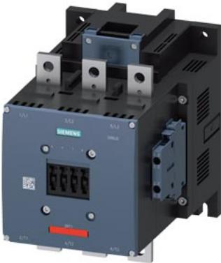
power contactor, AC-3e/AC-3 400 A, 200 kW / 400 V AC (50-60 Hz) / DC Uc: 220-240 V 3-pole, auxiliary contacts 2 NO + 2 NC permanently mounted drive: conventional main circuit: busbar control and auxiliary circuit: screw terminal
