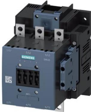
power contactor, AC-3e/AC-3 150 A, 75 kW / 400 V AC (50-60 Hz) / DC Uc: 110-127 V 3-pole, auxiliary contacts 2 NO + 2 NC drive: conventional main circuit: busbar control and auxiliary circuit: screw terminal
