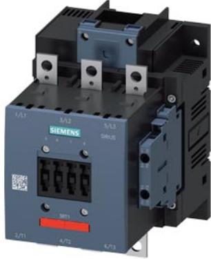
power contactor, AC-3e/AC-3 150 A, 75 kW / 400 V AC (50-60 Hz) / DC Uc: 110-127 V 3-pole, auxiliary contacts 2 NO + 2 NC permanently mounted drive: conventional main circuit: busbar control and auxiliary circuit: screw terminal
